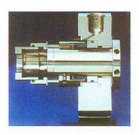
Due to the need for sealing rings to be impervious the carbon material is impregnated with either resin or various metals. VSK should be contacted to ensure the correct grade is used for the application. Seal faces can be supplied unlapped or if required lapped to two / three helium light brands of flatness.
